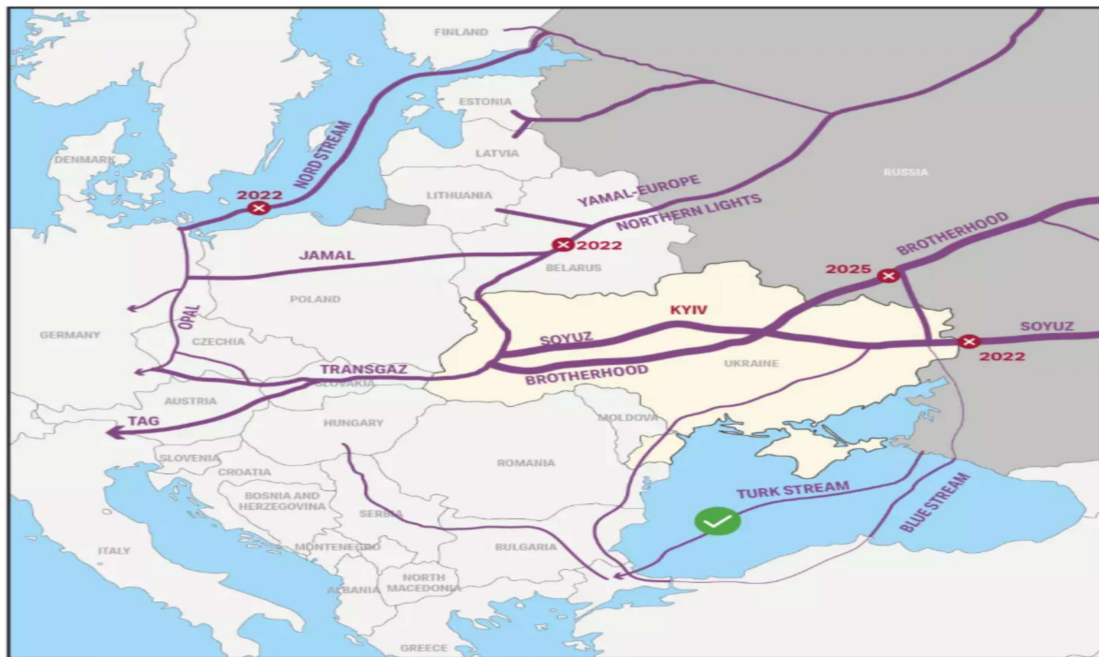
Figure 3 - Russian gas pipeline infrastructure in Europe
